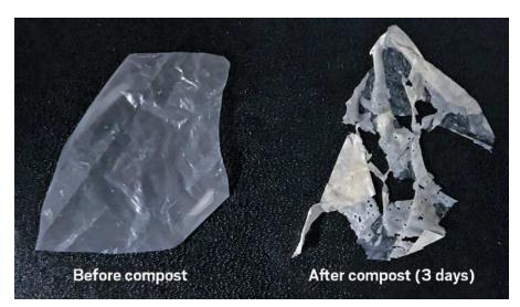
Encapsulated enzymes distributed throughout polycaprolactone can accelerate the breakdown of the material in the presence of heat and humidity. Photos show the material before and after composting for 3 days.
